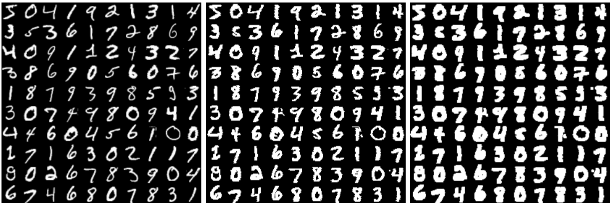
Figure 4: First 100 digits in the MNIST training dataset. Left: before deskewing. Center: after deskewing, without blurring. Right: after deskewing and blurring.
